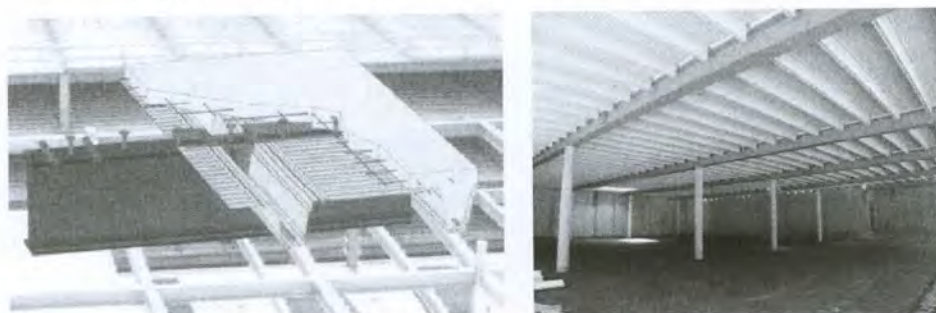
Fig. 5: Ribbed concrete floor in addition to the steel sheeting – system of Hoesch
